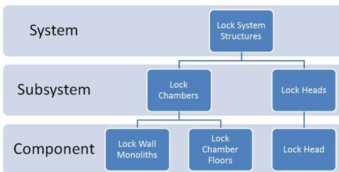
**Figure 2: Example SBS for Lock System Structures**
