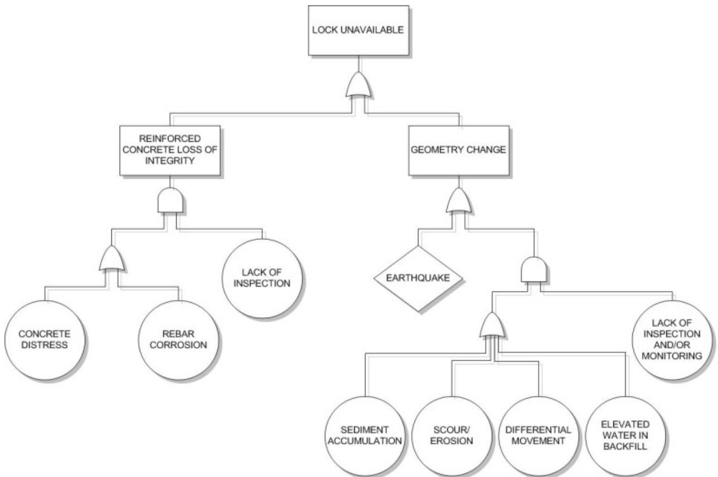
**Figure 3: Lock Chambers Conceptual Fault Tree Analysis**
