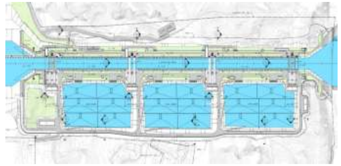
Figure 2: Three lift locks with nine water saving basins
