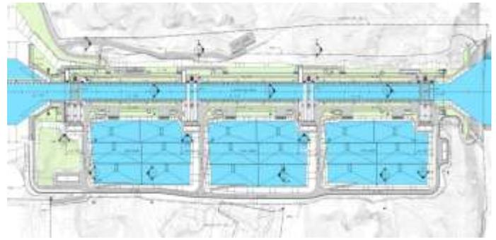
Figure 2: Three lift locks with nine water saving basins
