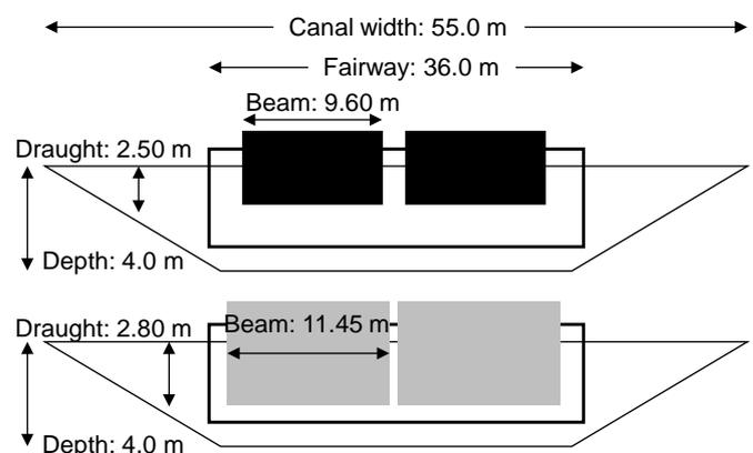
Figure 1: Design case Fairway width in canals
