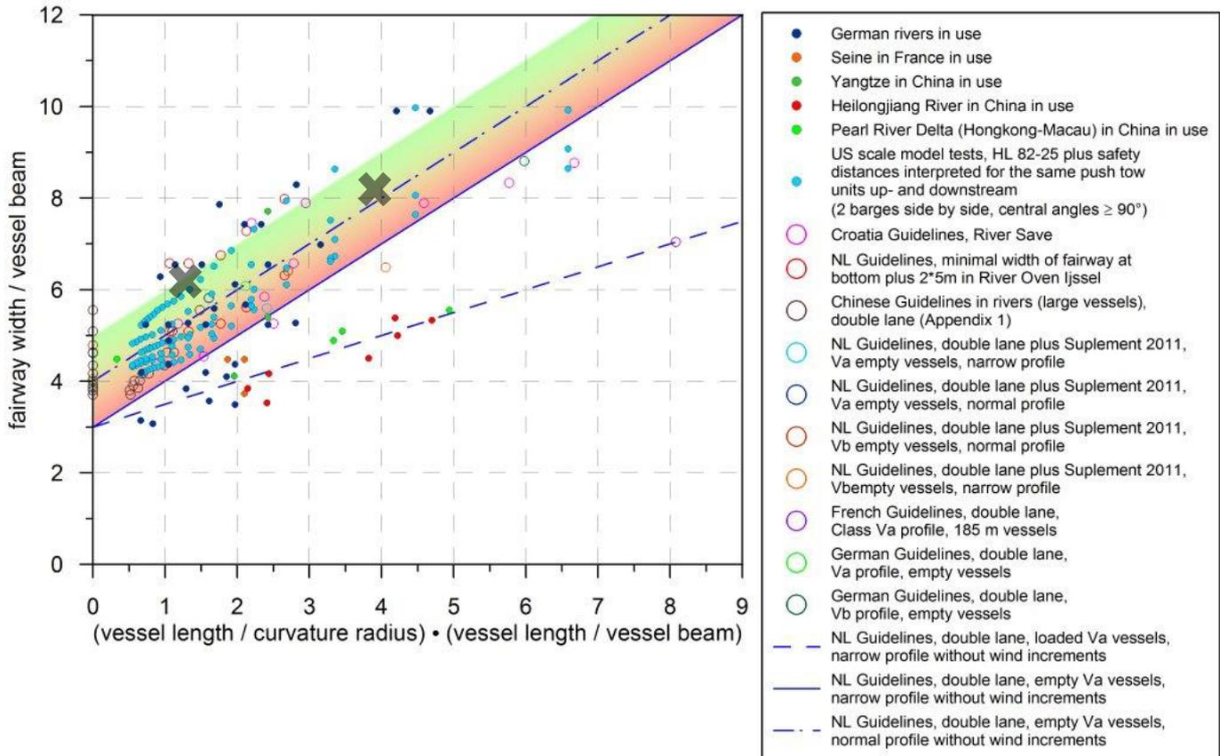
Figure 2: Existing fairway widths in rivers and from guidelines (width in draught depths), interpreted as to be limited by buoys, related to vessel breadth for two-lane traffic
