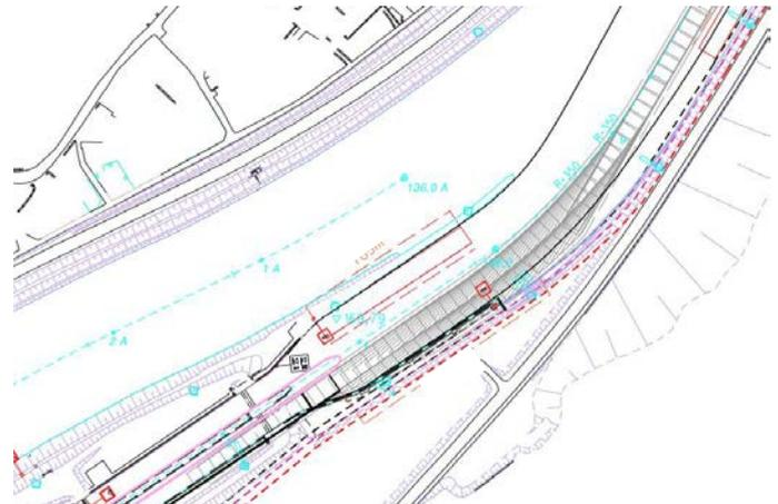
Figure 4: Detailed design lock approach (class Va vessel 110 m)
