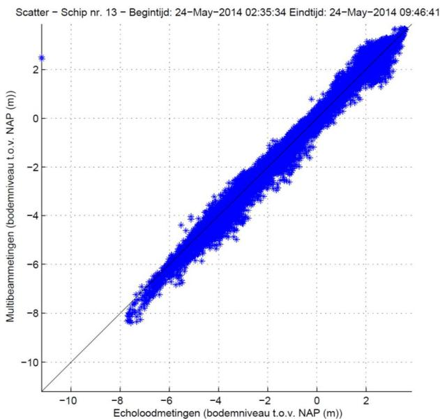
Figure 6: Example of scatter plot of COVADEM bed level versus Multibeam bed level.
