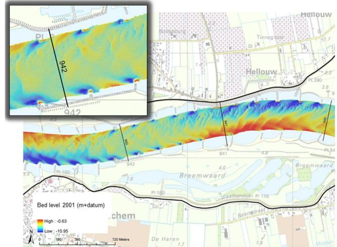
Figure 3: Example of a Rijkswaterstaat Multibeam data set. Morphological bend processes can be seen, as well as bedforms and ripples.
