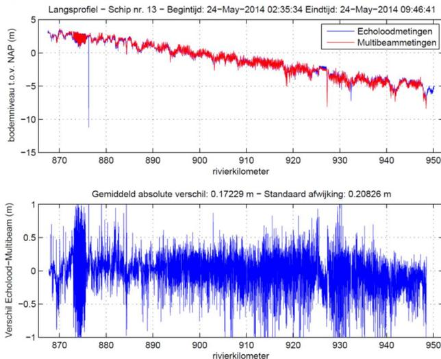
Figure 5: Example of longitudinal profile of measured bed levels; COVADEM bed levels in blue, Multibeam bed levels in red (top), and the difference between these (down).
