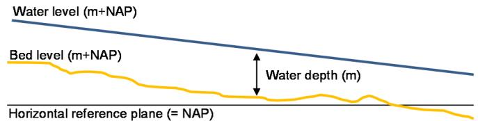
Figure 2: Definition sketch; note that both bed level and water level (and thus water depth) in rivers vary in time and space.
