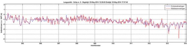
Figure 7: Example of a “good measurement”. Axes and legend as in Figure 5; on the horizontal axis distance in km, on the vertical axis bed level in m+NAP.
