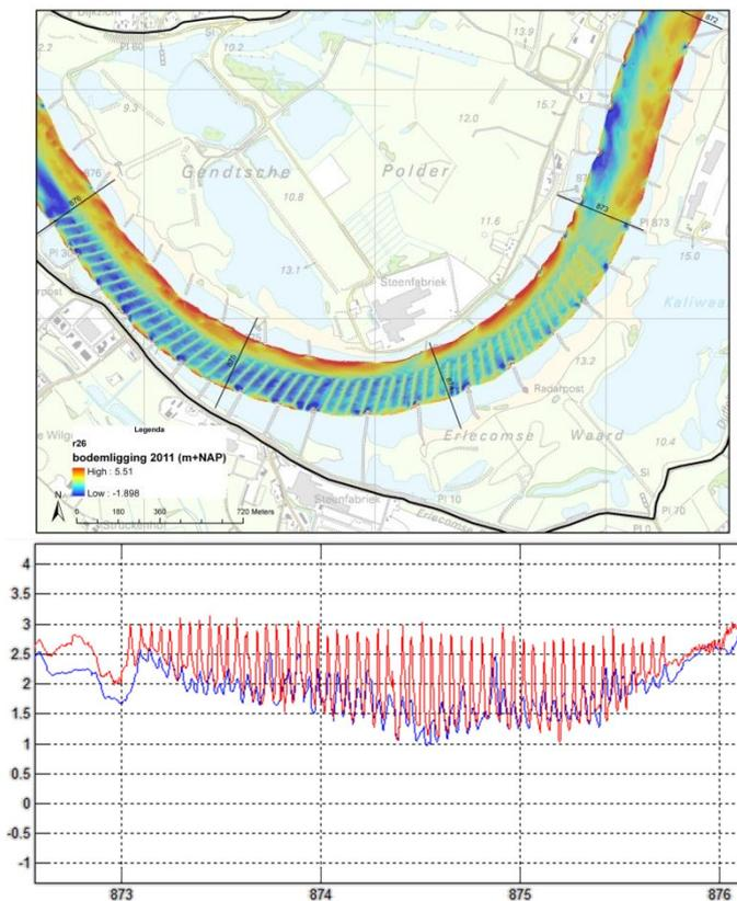
Figure 8: Bottom vanes at Erlecom. Axes and legend as in Figure 5; on the horizontal axis distance in km, on the vertical axis bed level in m+NAP.
