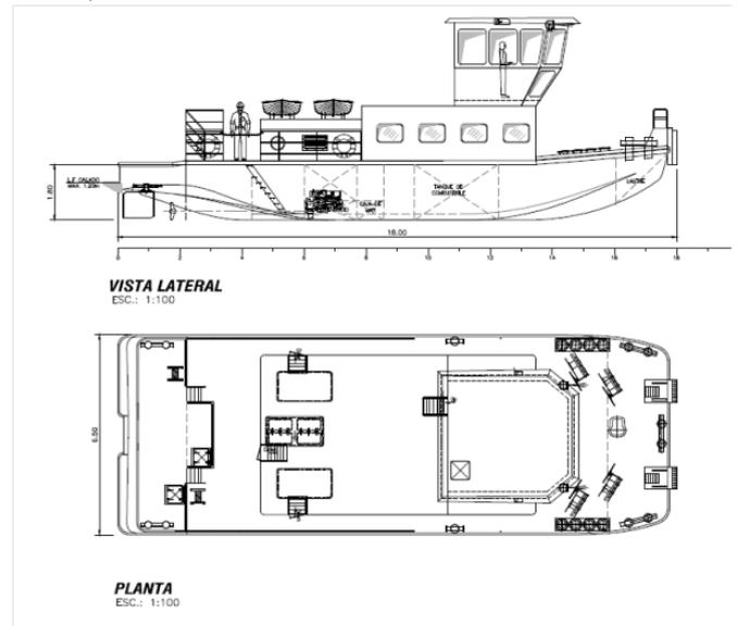
Figure 5: Dimensions of reduced pusher tug for Morona River
