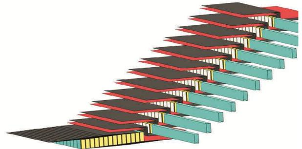
Figure 11: Pattern used to build up the foam and fibers onto the mold prior to resin injection (exploded view) [5].
