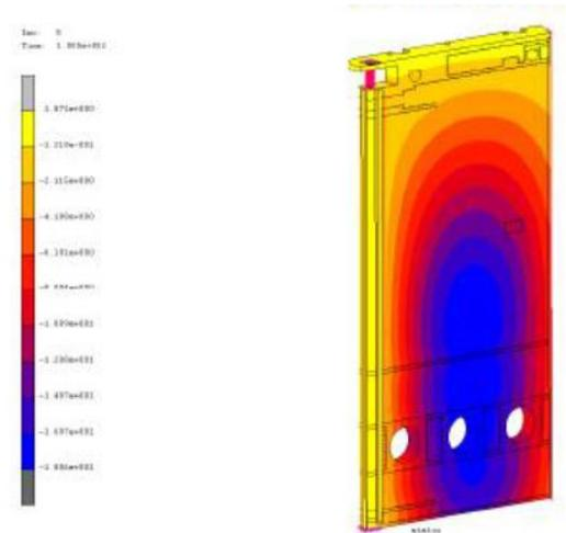
Figure 9: Calculated maximum deflection at SLS is 18 mm in the direction of the hydraulic load, at the vicinity of the structural beams.
