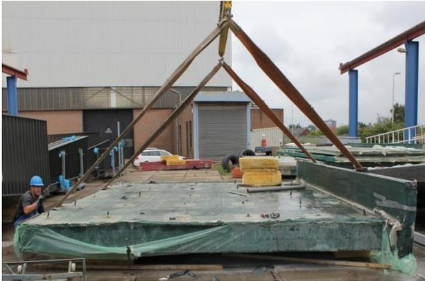
Figure 13: Semi-finished upper Gate leaf, 6.2 x 4.8 m. Manufactured by FiberCore Europe, Rotterdam, The Netherlands. Foil and runners still to be removed.
