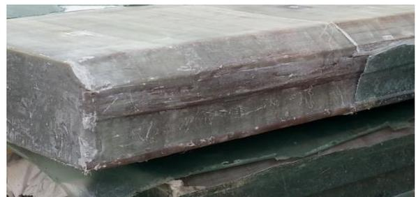
Figure 12: Mitre Gate leaf after curing and removing from the mold. All structural fiber elements have become a one-piece FRP composite structure.
