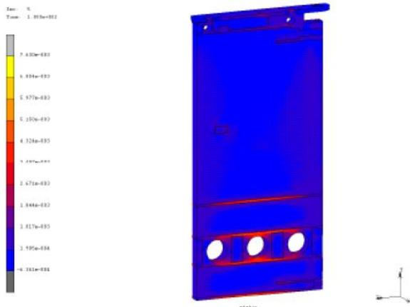
Figure 10: Calculated maximum principle strain is 0.76% at ULS in the vicinity of the structural beams.
