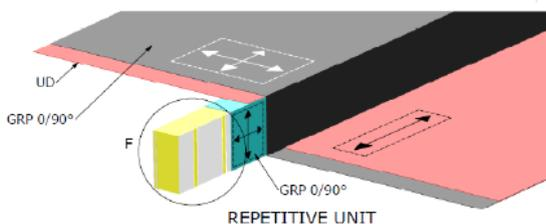
Figure 7: The Z-shaped continuous fiber and foam build-up used in the FRP Composite Mitre Gates.
