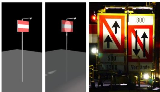
To ensure that the colours of the signs are not falsified by the illumination, the required colour temperature of the LEDs should be approx. 4000 K (neutral white).
