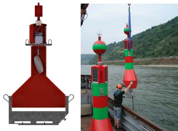
Figure 5: Standard PE oval buoy with lantern, solar power box and integrated radar reflector, positioning of the 335 kg buoy
