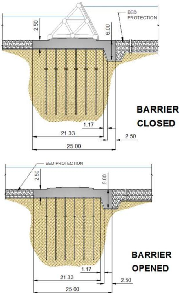
Figure 14: Preliminary Foundation Design for Steel Barrier
