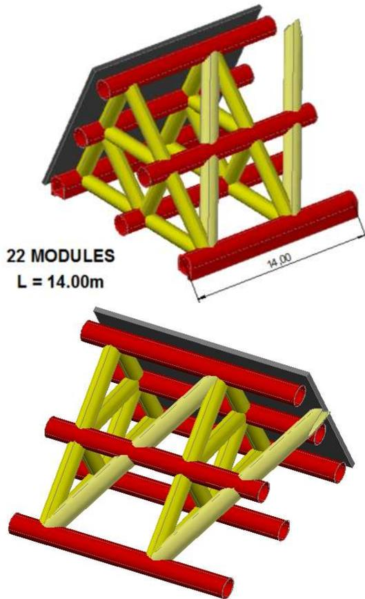
Figure 9: Main Barrier Design: Steel and Concrete
