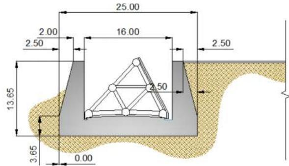
Figure 15: Chamber for Steel Barrier (Foundation piles not pictured)
