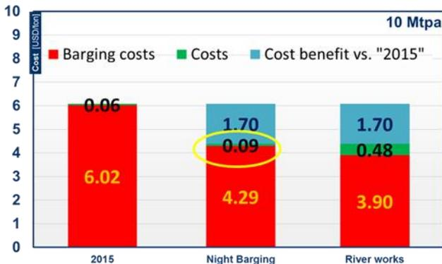
Figure 10 Cost reduction of implementing night barging or river works in USD/t coal transported from Muara Lematang to a sea going vessel offshore. The cost figures are for 10 Mtpa export of coal.
