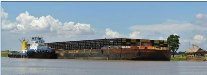
Figure 4: Top RoRo barges. Second: 7,500 DWT barge passing Ampera Bridge in Palembang. Third: Bridge passing upstream Musi River section. Bottom: Musi River typical 7,500 DWT barge and 2400 Hp tug combination parked and waiting for being loaded.
