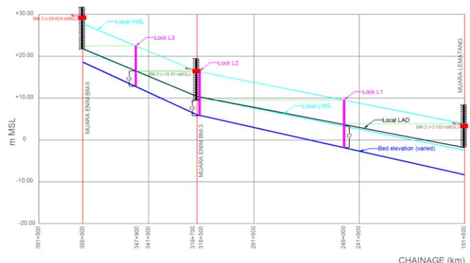
Figure 11 River cross section with indicative locations of ship locks to manage the water level in the dry season.
