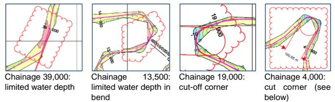
Figure 2: Bend radius calculations from bathymetries
