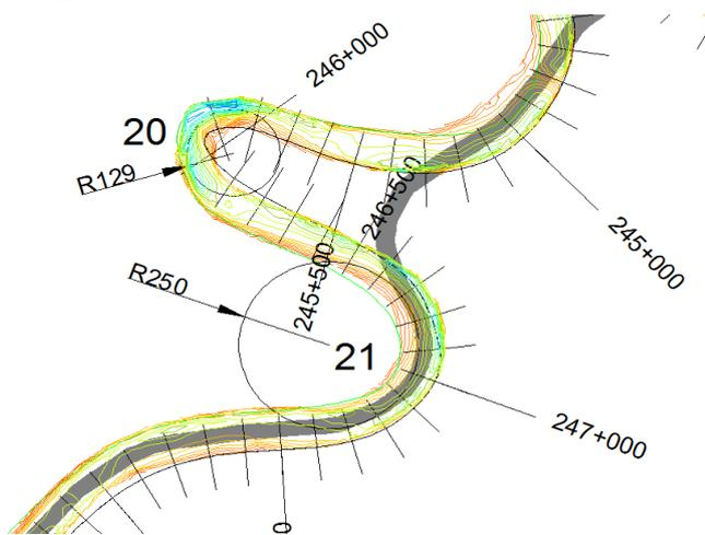
Figure 12: Example of the total of 32 bend cuts to be made on the Lematang River.
