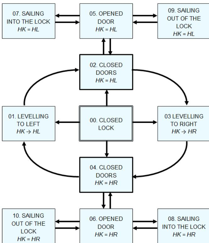
Figure 7: The generic functional diagram on which the locking procedure is based. The arrows between phases denote the conditions to be met before a transition to the next phase.
