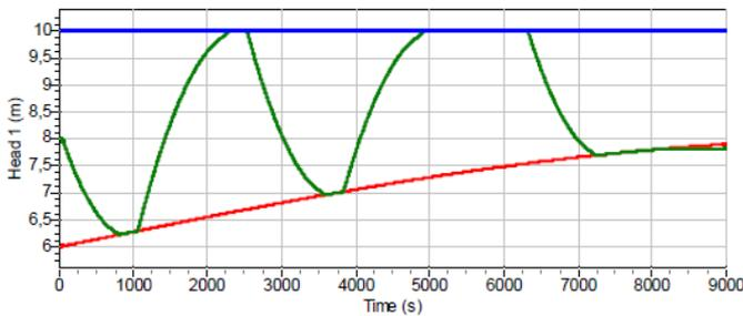
Figure 5: The timeseries of water levels in the approach harbours (blue, red) and lock chamber (green), resulting from a simulation with a predefined schedule of valve openings. The locking sequence can be recognized in the raising and lowering of the lock chamber’s water level.
