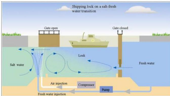
Figure 2: Salt intrusion mitigating measures in a shipping lock on a salt-fresh water transition. From Keetels et al. (2011).
