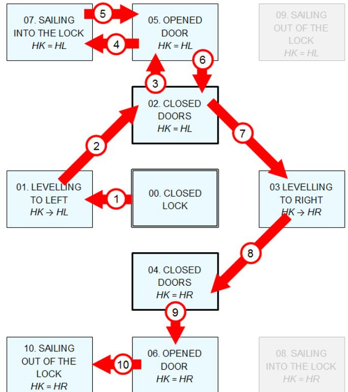
Figure 8: The sequence of actions in order to realize a lockage from left to right, as described in Section 5.6.
