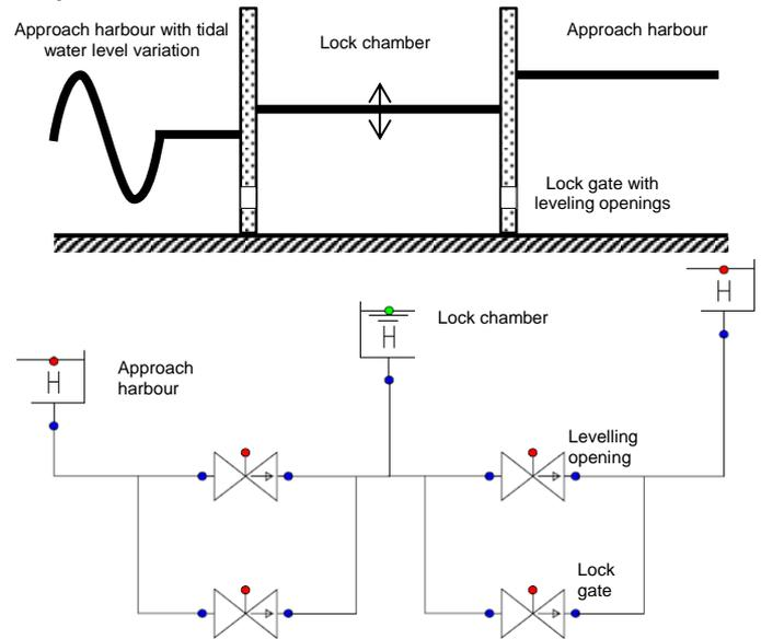
Figure 3: An illustration of a simple shipping lock with lock gate openings (top) and its representation using WANDA components (bottom).
