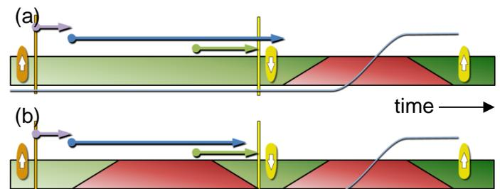
Figure 6: Closing the door after the sailing out following a lockage, before the sailing into the lock for the subsequent lockage.
