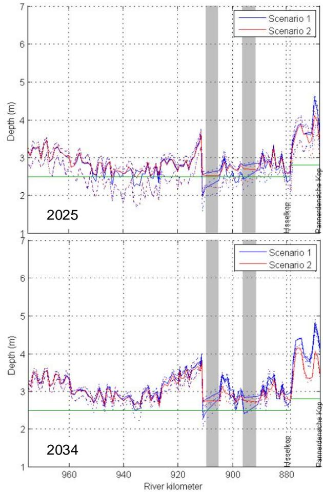
Figure 9: 10<sup>th</sup> percentile of the depth with respect to ALW per kilometre block in the Pannerdensch Kanaal and IJssel, the shaded areas denote jumps in the river kilometres, caused by former bend cut-offs. The green line denotes the maintenance depth.
