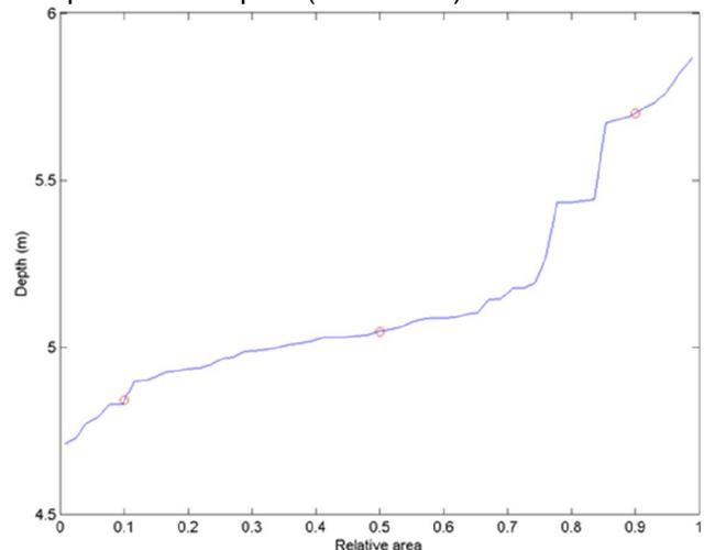
Figure 7: Depth distribution as function of the relative area in the navigation channel.
