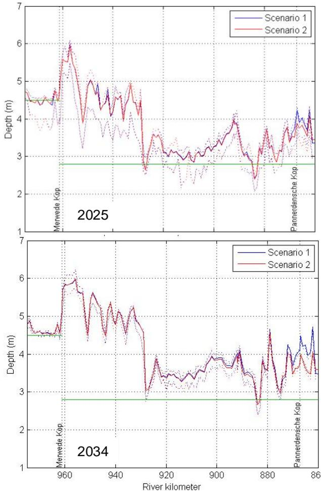
Figure 8: 10<sup>th</sup> percentile of the depth with respect to ALW per kilometre block in the Bovenrijn, Waal, and Nieuwe Merwede. The green line denotes the maintenance depth.
