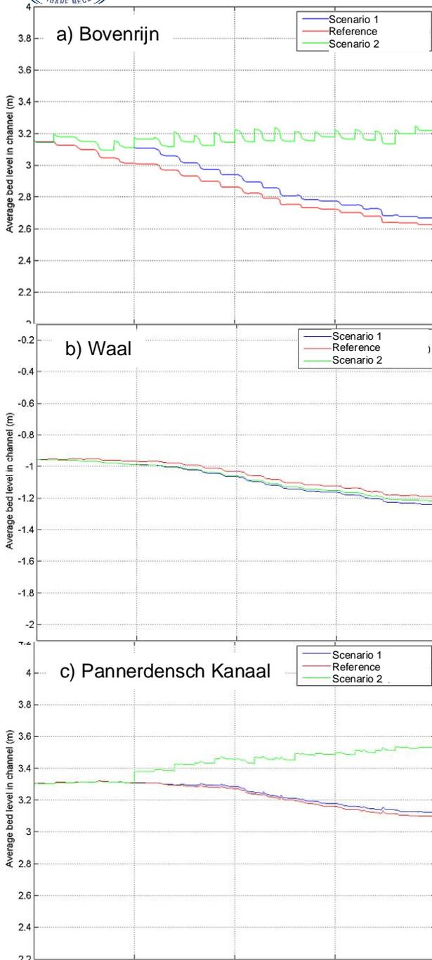
Figure 5: Average bed level for different river reaches for the different cases.
