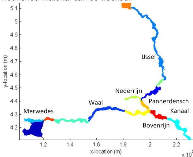
Figure 2: Overview of the 12 computation domains used in the hydro-morphodynamic computations.
