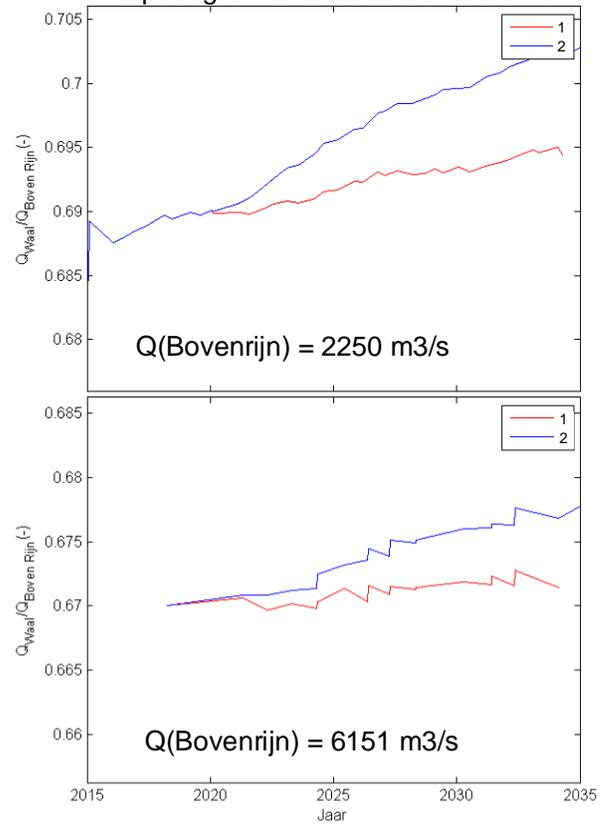
Figure 6: Ratio of the discharge flowing the Waal at the Pannerdensch Kop at low and high discharge levels.
