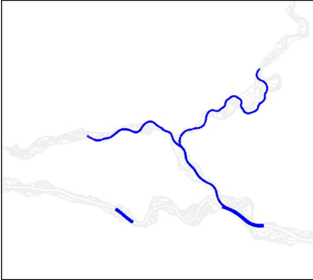
Figure 3: Areas considered for yearly bed stabilisation from 2020 onwards in the Bovenrijn, Pannerdensch Kanaal, IJssel (first 40 rkm), Nederrijn and behind the fixed layer at Nijmegen.
