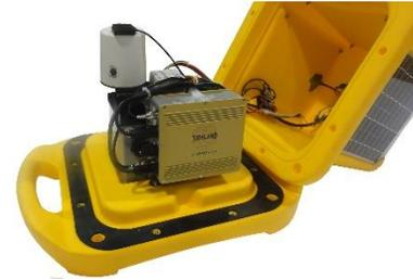
**Figure 3- AIS fitted within a self-contained lantern**
