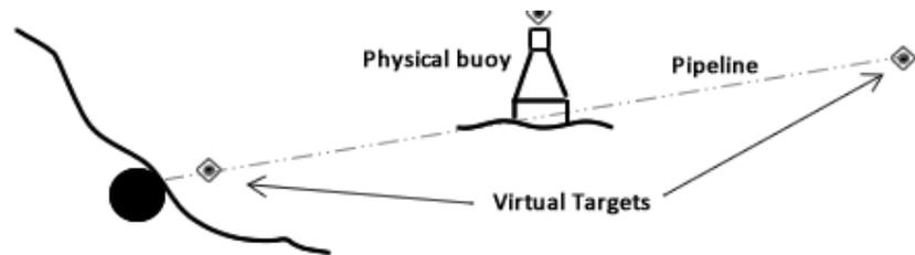
**Figure 7- Pipeline marker with virtual AIS**
