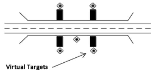
**Figure 6- Bridge marked by real and virtual AIS**
