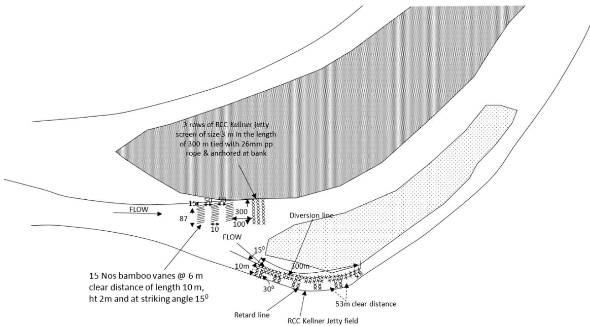
Figure 1-(B): Detail Arrangement of Location (B) At Nakhwa Site (Ch 1299)
