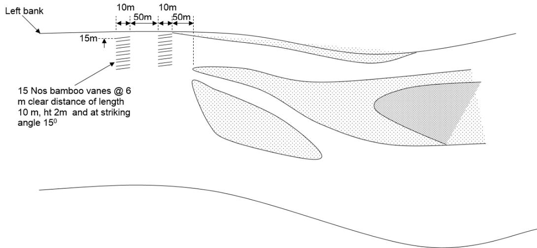
Figure 1-(A): Detail Arrangement of Location (A) At Nakhwa Site (Ch 1299)
