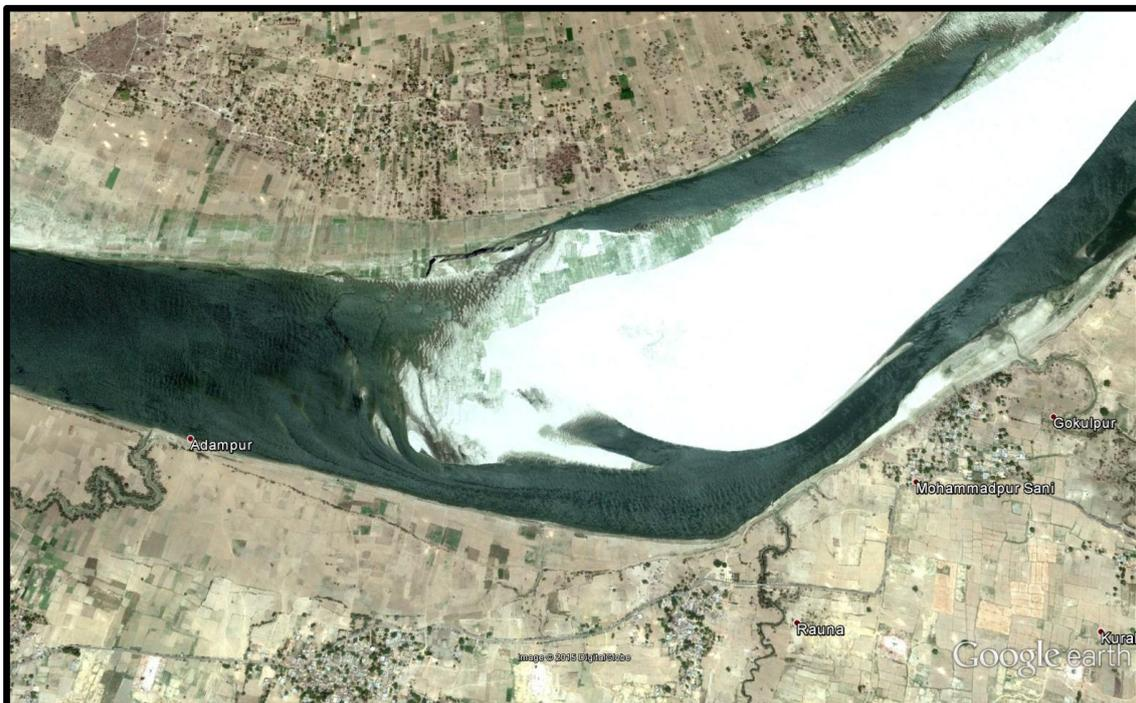
Figure 4: Satellite Image March 2012 of Ganga River for Post Jack Jetty Installation near Nakhwa Village (12KM D/S of Varanashi)
