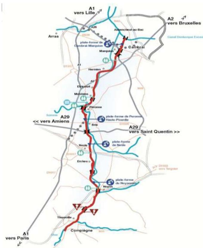
Covering a total land area of 2,450 ha (facilities included), the 107 km long-, 54 m wide- and 4.5 m deep-canal will run from Compiègne to Aubencheul-au-Bac. It will include 6 locks, 61 road- and railway-bridges, 3 aqueducts and 1 storage reservoir. It is also planned to build 4 multimodal platforms, 5 grain quays, 2 transshipment quays and 5 boat moorings.
