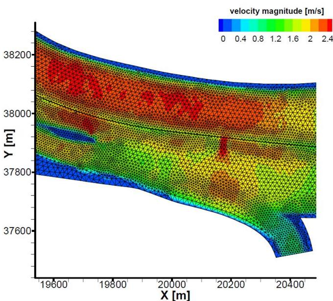
Figure 1: CFD simulation for the German river Rhine at 530 km.
