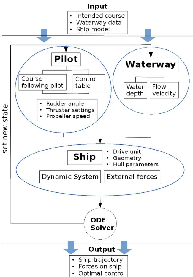
Figure 4: Simulation work flow of FaRAO
