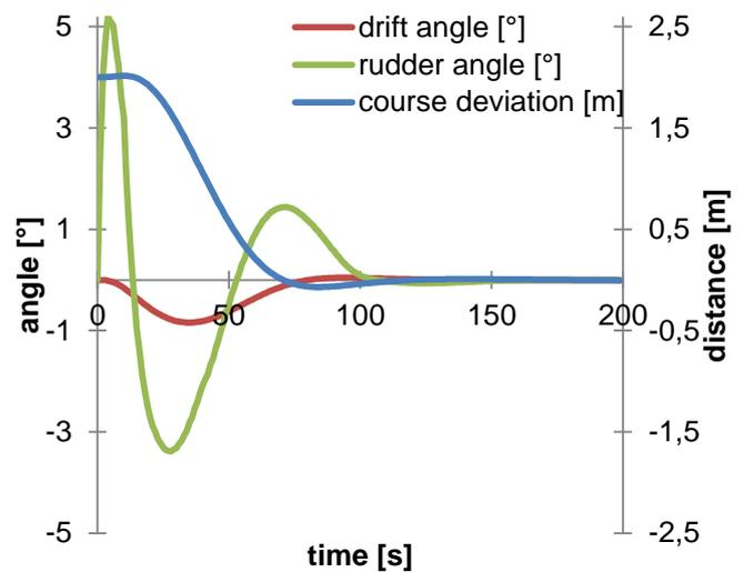
Figure 6: Ship performing a lateral offset maneuver controlled by the course following pilot
