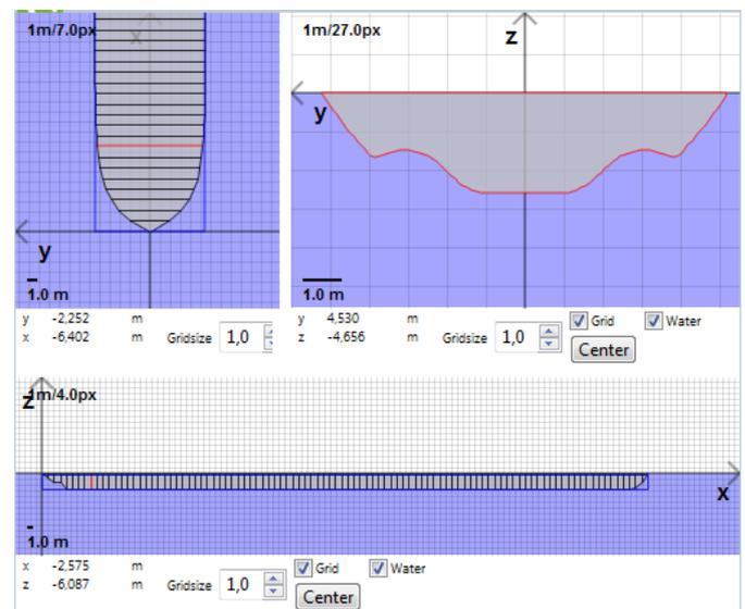
Figure 2: The tool HULK developed at the BAW to import ship models for FaRAO.
