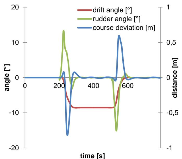
Figure 7: Ship sailing through cross flow field controlled by the course following pilot.
