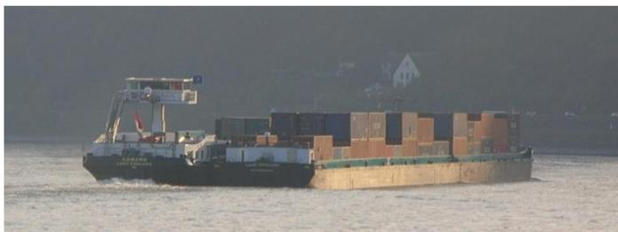
Figure 2: Self-propelled container vessel with three barges at low water level on the Rhine.
