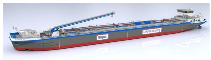
Picture 6: Combined LNG/MGO tanker of Argos Bunkering
