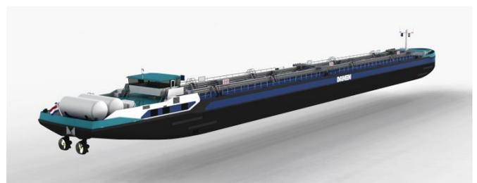
Picture 5: 100% LNG fuelled inland chemical tanker “Ecoliner” of Damen
