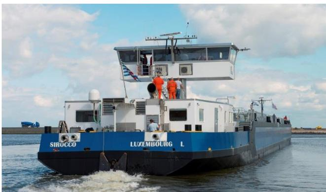
Picture 3: LNG fuelled inland chemical tanker “Sirocco” of Chemgas Barging
