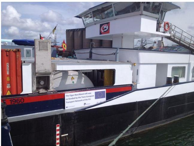
Picture 2: Retrofitted dual-fuel container vessel “Eiger” of DCL Barge
