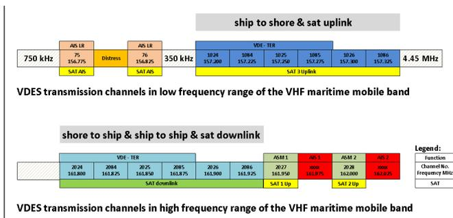
Figure 2: Example of channel designation for VDES in the VHF maritime mobile band.
