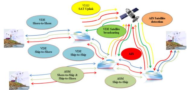
Figure 1: VDES functions for data exchange between ships, shore and satellite.
