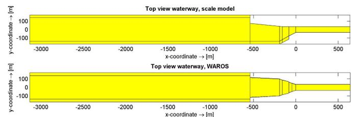
Figure 1: Upper: Waterway layout of the IJmuiden scale model tests. Lower: Symmetrical waterway schematization of WAROS.
