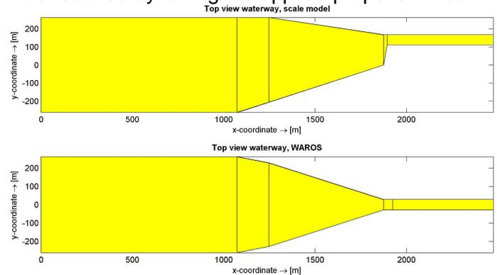
Figure 6: Upper: Waterway layout of the Zeebrugge scale model tests. Lower: Symmetrical waterway schematization of WAROS.
