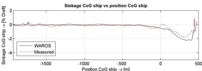
Figure 3: Resulting sinkage of the CoG of the ship of the IJmuiden scale model test 029.
