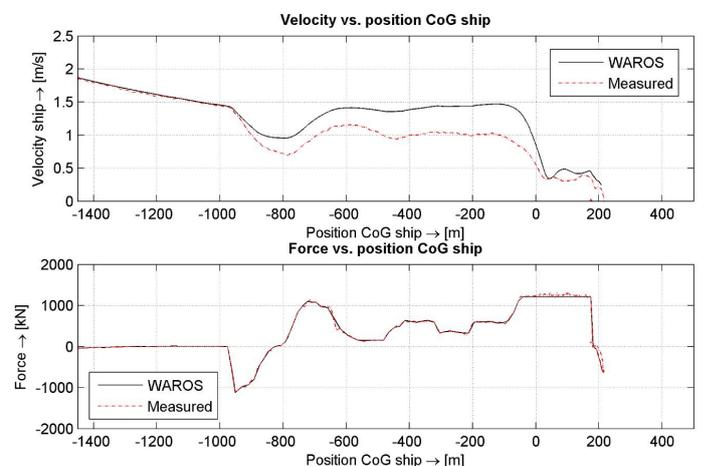
Figure 5: Resulting ship velocity (upper) and forces on the ship (lower) of the Panama scale model test B.
