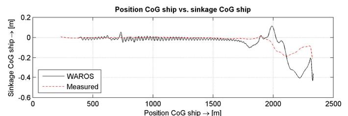
Figure 8: Resulting sinkage of the CoG of the ship of the Zeebrugge scale model test G.
