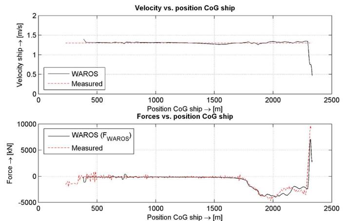
Figure 7: Resulting ship velocity (upper) and resistance forces on the ship (lower) of the Zeebrugge scale model test G.
