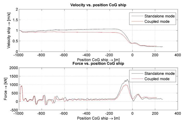
Figure 11: Coupled and standalone results of cond02 with a constant propeller thrust.
