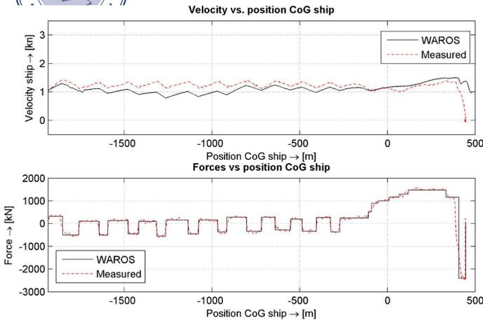
Figure 2: Resulting ship velocity (upper) and forces on the ship (lower) of the IJmuiden scale model test 029.
