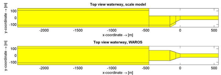
Figure 4: Upper: Waterway layout of the Panama scale model tests. Lower: Symmetrical waterway schematization of WAROS.
