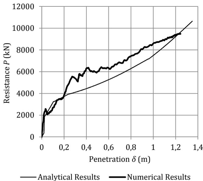
Figure 13: Numerical and analytical results for an impact by a conventional bow
