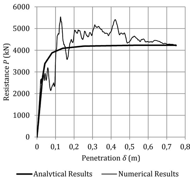
Figure 14: Numerical and analytical results for an impact by a river barge
