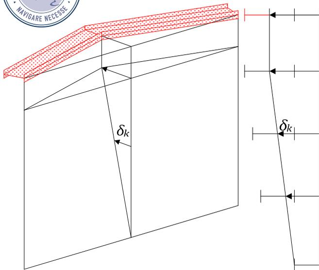
Figure 9: Beam model and displacement field during the global deforming mode
