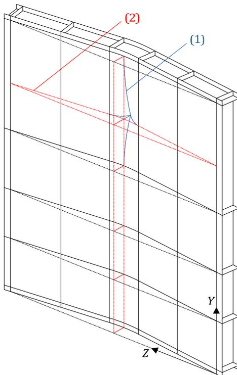
Figure 5: Local and global deforming modes
