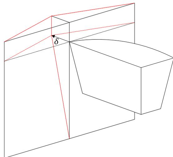
Figure 8: Global bending motion of the gate
