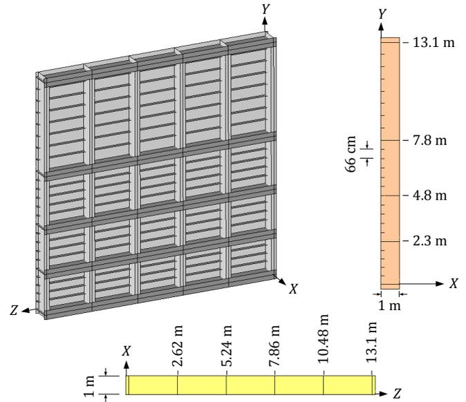
Figure 10: Lock gate used for validation
