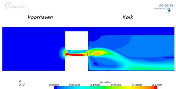
Figure 14: Vertical cross-section: water velocity magnitude with the door valve half open; leveling with density differences
