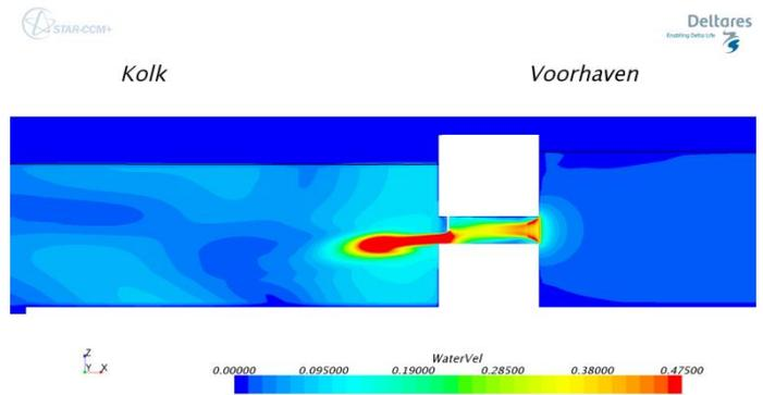
Figure 17: Vertical cross-section: water velocity magnitude with the door valve half open; leveling without density differences
