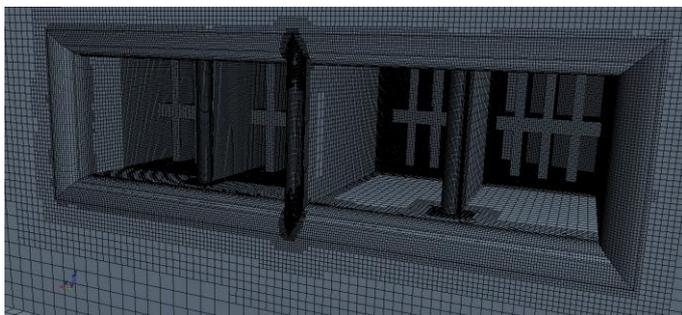
Figure 9: View of the surface mesh of the mouth of the culvert
