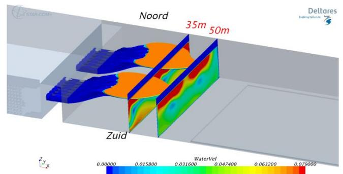
Figure 13: Isosurface of velocity, coloured by water level; plus, vertical cross-sections of water velocity magnitude contours at the stop lines. Door valve is half open; leveling without density differences
