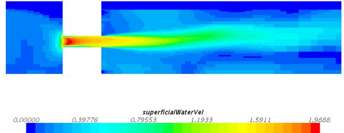
Figure 7: Contour plot of water velocity magnitude of the door valves without breaking bars
