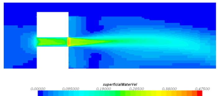
Figure 8: Contour plot of water velocity magnitude of the door valves with breaking bars
