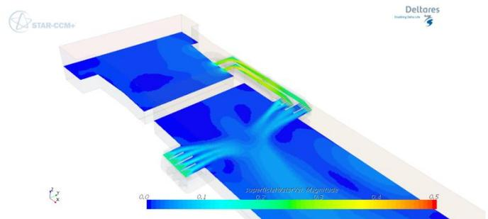
Figure 11: Contour plot of the water velocity magnitude for the culverts at the western lock head.
