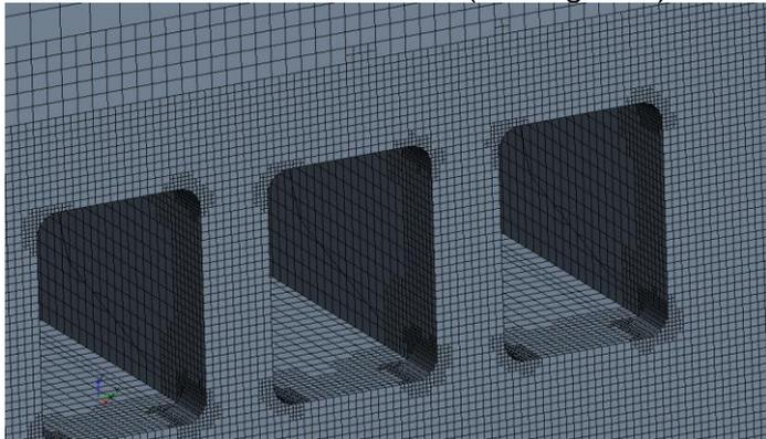
Figure 5: View of the surface mesh of the gate openings without breaking bars
