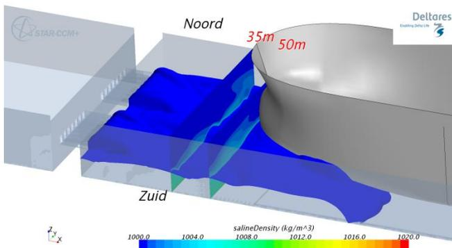
Figure 23: Isosurface of salt concentration; plus, vertical cross-sections of water density contours at
