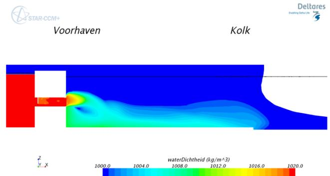
Figure 20: Vertical cross-section: water density with the door valve half open; leveling with density differences, before reflection against bow
