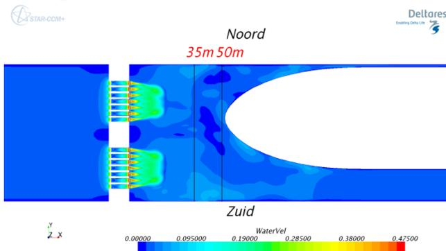
Figure 19: Horizontal cross-section: water velocity magnitude with the door valve half open; leveling with density differences
