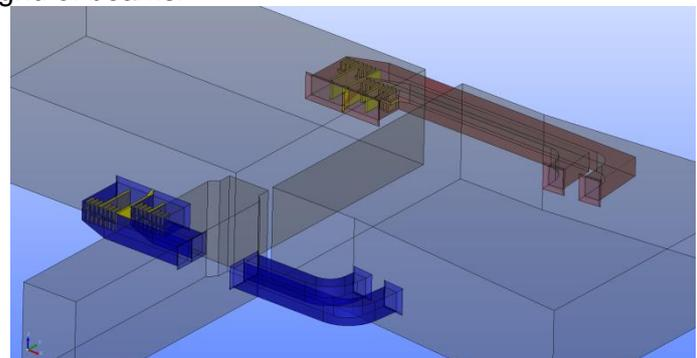
Figure 3: Geometry with culverts eastern lock head
