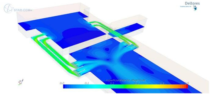
Figure 10: Contour plot of the water velocity magnitude for the culverts at the eastern lock head.
