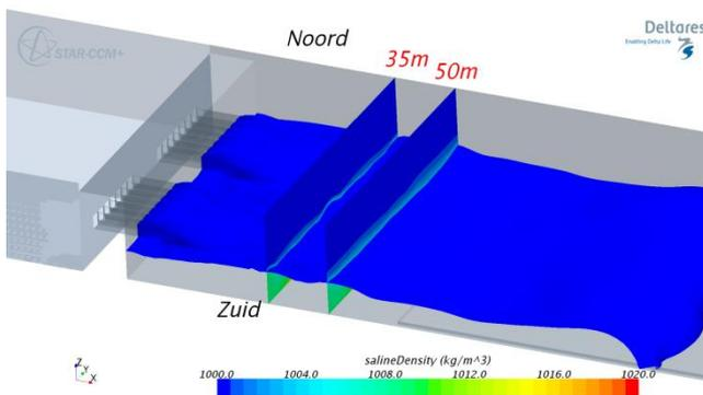
Figure 16: Isosurface of salt concentration; plus, vertical cross-sections of water density contours at the stop lines. Door valve is half open; leveling with density differences
