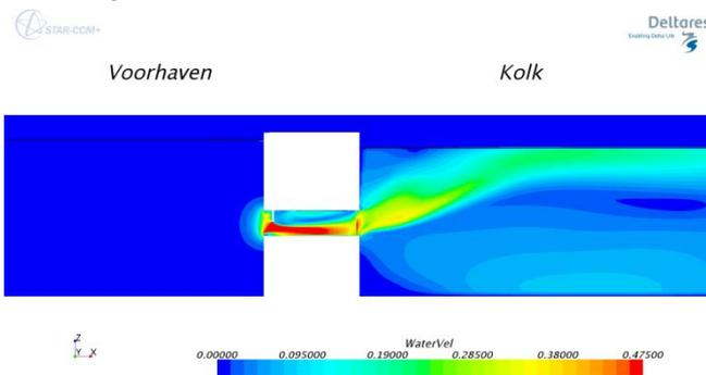
Figure 12: Vertical cross-section: water velocity magnitude with the door valve half open; leveling without density differences
