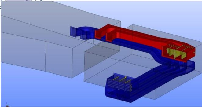
Figure 4: Geometry with culverts western lock head
