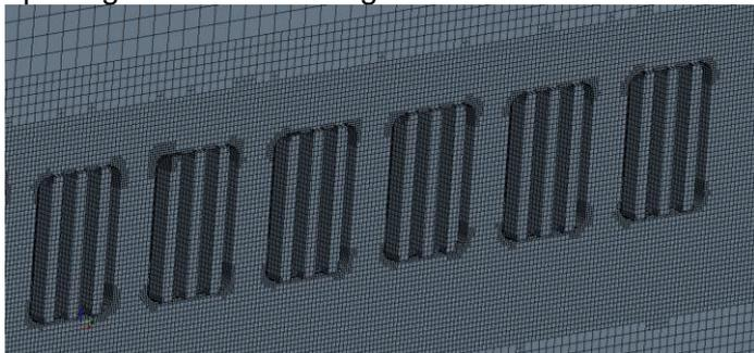
Figure 6: View of the surface mesh of the openings with breaking bars
