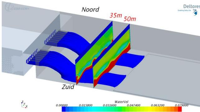
Figure 15: Isosurface of velocity, coloured by water level; plus, vertical cross-sections of water velocity magnitude contours at the stop lines. Door valve is half open; leveling with density differences
