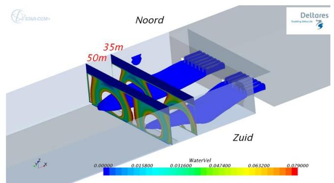
Figure 18: Isosurface of velocity, coloured by water level; plus, vertical cross-sections of water velocity magnitude contours at the stop lines. Door
