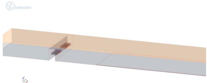
Figure 2: Geometry with gate openings, the approach harbor is on the left and the lock chamber is on the right
