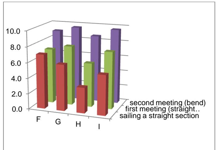
Figure 9: Standard deviation of the rudder angle [deg]
