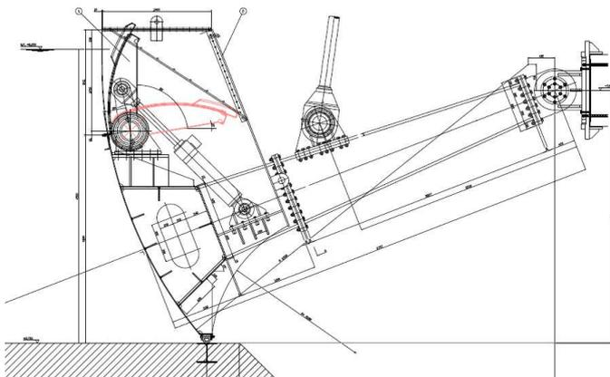
Figure 2: cross-section of the tainter gate with flap
