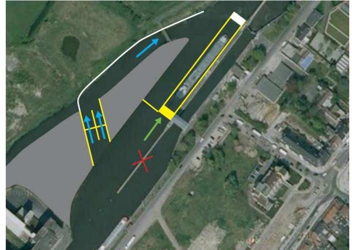
Figure 9: Temporary weirs and lock
