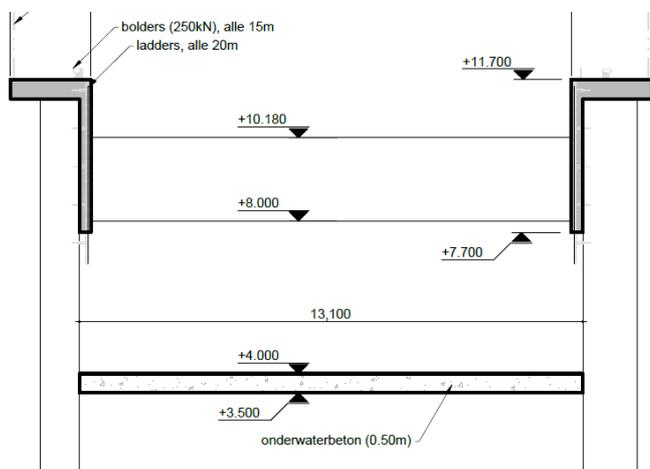
Figure 8: Cross-section of the temporary lock
