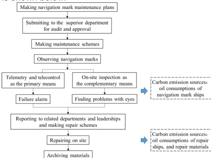
Figure 3: Workflow and carbon emission sources of the existing mode of navigation mark maintenance
