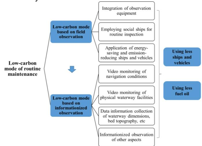
Figure 2: Low-carbon mode of routine maintenance observation
