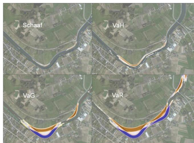
Figure 1: Example of the spatial effect of the 4 alternatives on the morphology in the Hoogland Bend. The impact of VaH is smaller than in VaG or VaR because no cutting or axial translations are allowed in VaH. The double lane functionality in VaR requires changes to nearly the complete
