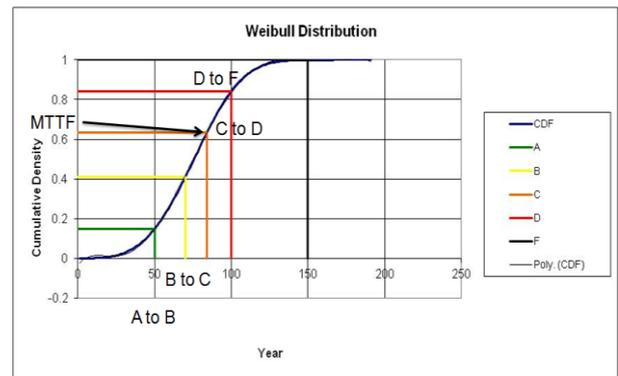
Figure 4 Mapping of Condition to Weibull CDF
