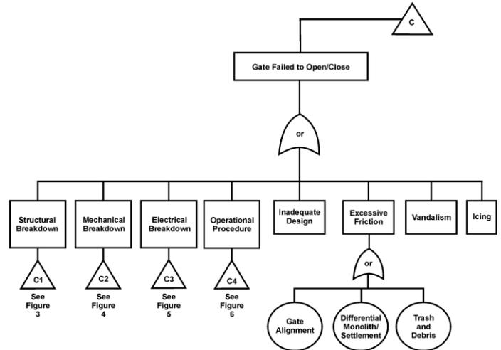
Figure 8 – Example Fault Tree for Dam Gate (Patev and Putcha 2005)
