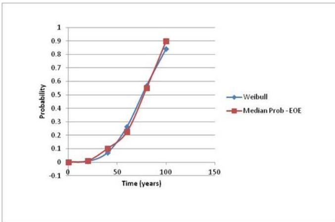
Figure 2 Example of Weibull Curve
