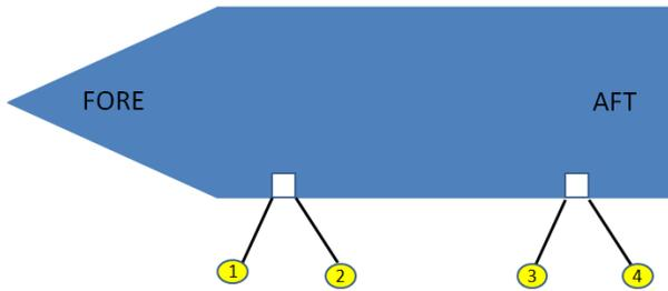
Figure 1: Four Mooring Wires are required for lockages
