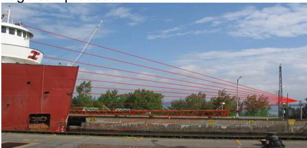
Figure 7: Laser Scanner to spot vessel into lock
