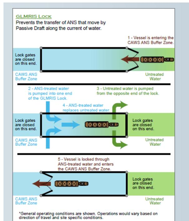
Figure 6: Vessel Passing through GMRIS Lock
