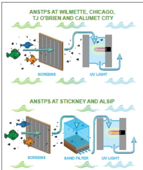
Figure 8: Treatment Plant Process
