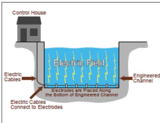
Figure 7: GLMRIS Electric Barrier Layout
