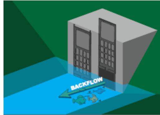
Figure 9: Screened Sluice Gates
