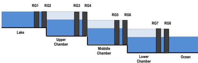
Figure 2 – Numbering of the Rolling gates scheme
