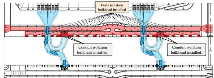
Figure 10 – Scheme for a Special operation with WSBs and with one Culvert in dry condition
