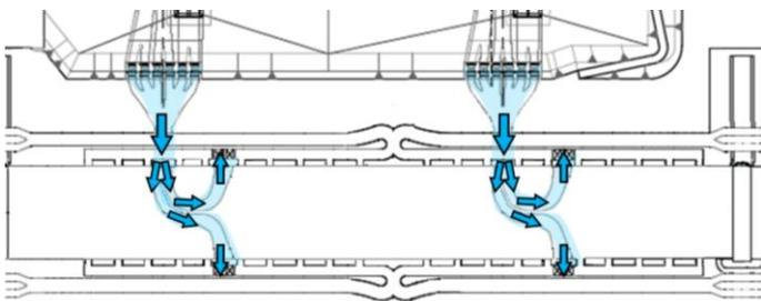
Figure 9 – Scheme showing the flow split symmetrically between the two secondary culverts
