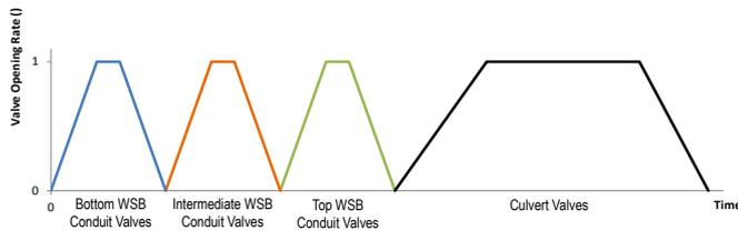
Figure 7 –Valves schedule scheme for a chamber filling
