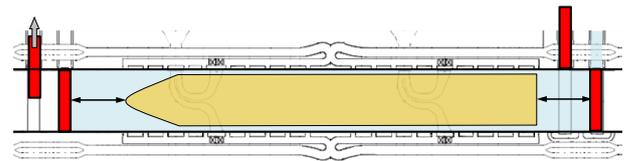
Figure 3 – Scheme for Uplockage Standard Chamber configuration
