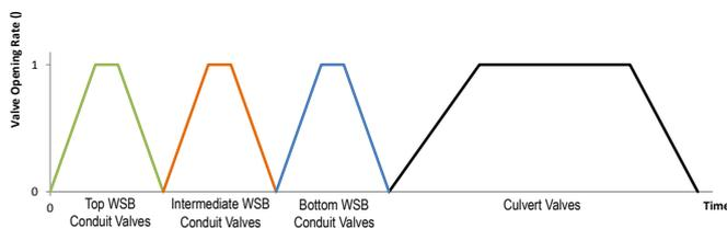
Figure 8 –Valves schedule scheme for a chamber emptying
